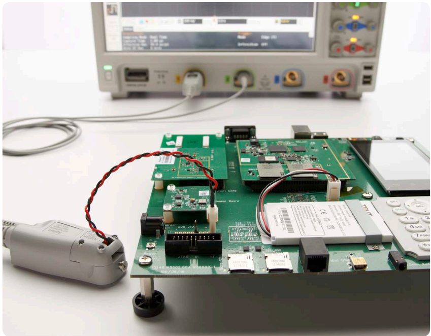
Figure 1. Agilent's ultra sensitive N2820A/N2821A current probes (with resolution as low as 50 \mu A) excel at measuring for small current levels typically found in battery powered devices.
