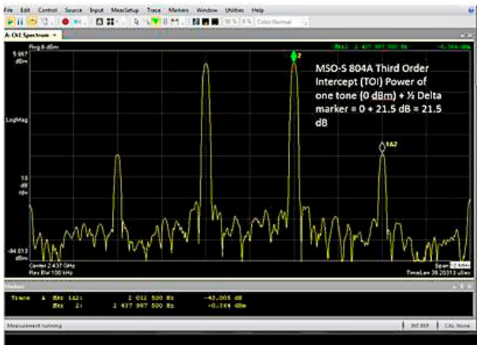
Using data acquired from S-Series, VSA shows an excellent TOI value of 25 dBm.
