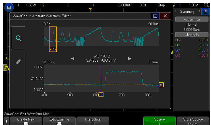
Figure 26. Optional arbitrary waveform generator provides easy access to stimulus. The integrated arbitrary waveform generator makes capturing, modifying and replaying signals simple.
