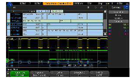
Figure 19. Multi-bus time aligned decode.
