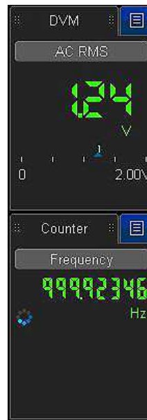
Figure 27. DVM and counter takes advantage of separate signal paths to provide measurements without a trigger, while still using the scope probes.
