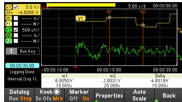
Figure 7. Log data with sample interval 20 \mu s to 60 s, for up to 10,000 hours or 5 MB of data
