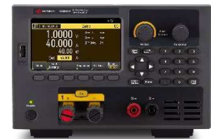
Figure 1. EL33133A 250 W bench electronic load 150 V, 40 A
