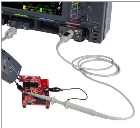
Figure 14. CX1151A passive probe interface adapter
