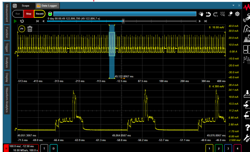
Figure 19. CX3300 can read and playback from the storage for deep analysis similar to the scope mode
